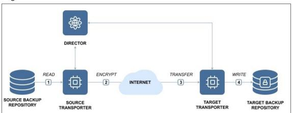
If you plan to transfer data over WAN without a VPN connection from your source site to the target site, make sure the source and target **Transporters** are added to the product using external IP addresses or DNS names that can be properly resolved in WAN, so that the two **Transporters** can connect to each other.
