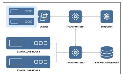
Deploying multiple **Transporters** also enables network acceleration and AES 256 encryption of traffic between a pair of **Transporters**. For example, if VMs are replicated over WAN between two sites, the **Transporter** installed in the source site can compress and encrypt data before transferring it over WAN, and the **Transporter** installed in the target site can unencrypt and decompress the data prior to writing it to the target server.
