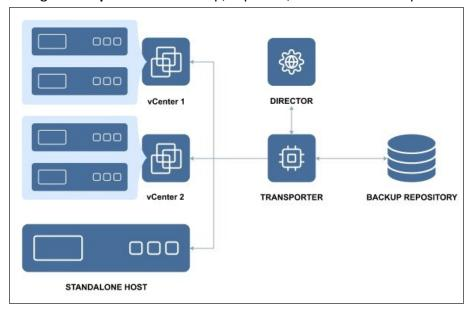
One Transporter can simultaneously process multiple source disks (6 by default) during backup, replication, and recovery. If jobs contain more disks than the **Transporter** is set to process simultaneously, the disks will be put in a queue and will be processed once the **Transporter** frees up.
