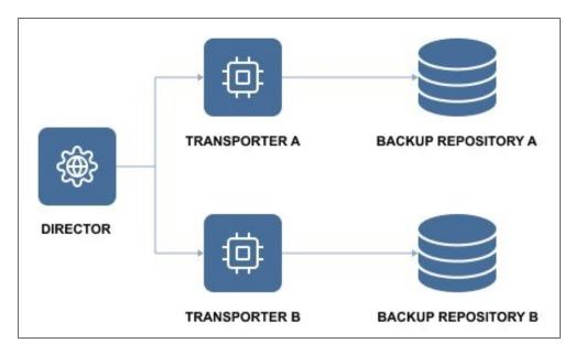
The Assigned **Transporter** is responsible for all interaction with its **Backup Repository**. A single **Transporter** can be assigned to and manage multiple **Backup Repositories**.
