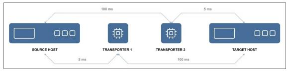
In the example above, **Transporter** 1 will be selected to read data from the Source ESXi, and **Transporter** 2 will be selected to write data to the Target ESXi.
