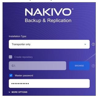
3. Optionally, you can select the **Master password** checkbox and enter the password that will be used to generate a pre-shared key and secure the **Transporter**.
